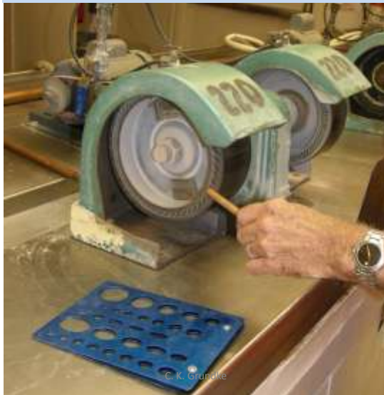
Using Dop Stick to Center Belt on Wheel as it slows down.
