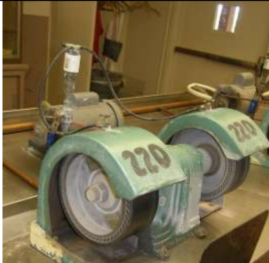
Final shaping process using 220-400-600 sanding belts to remove flat spots.
